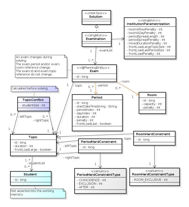
Figure 3.3. Examination Domain Class Diagram
