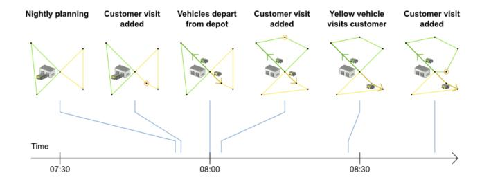
In the example above, three customers are added at different times (07:56, 08:02 and 08:45), after the original customer set finished solving at 07:55, and in some cases, after the vehicles already left.
