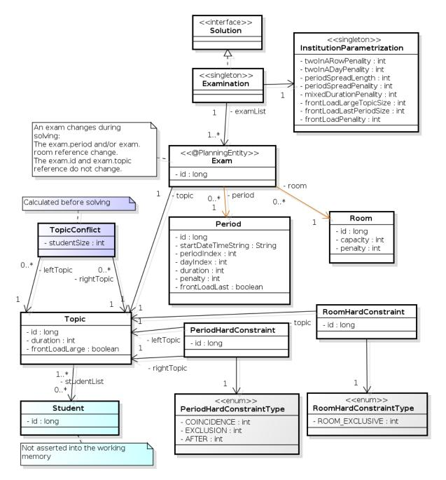
Figure 3. Examination Domain Class Diagram
