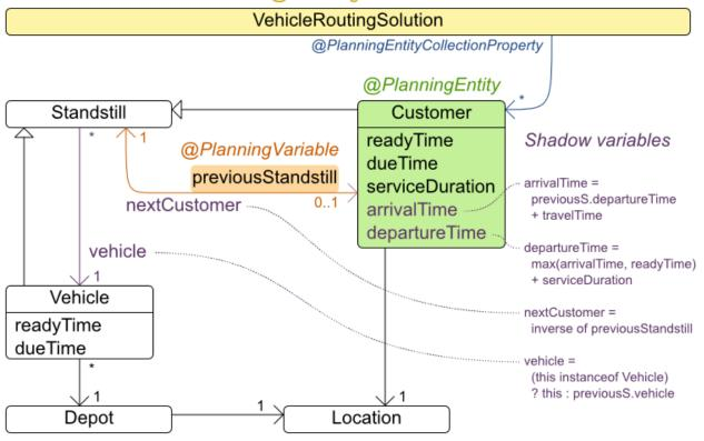
The vehicle routing with timewindows domain model makes heavily use of shadow variables. This allows it to express its constraints more naturally, because properties such as arrivalTime and departureTime, are directly available on the domain model.
